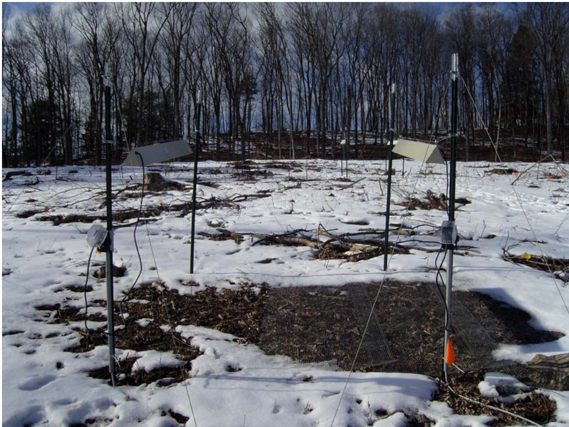
Figure 1. Two Kalglo infrared heating lamps suspended over one of eight 2X4m plot being experimentally warmed at our research site in central PA. This picture was taken a few days after heating was initiated in late winter, 2008.
